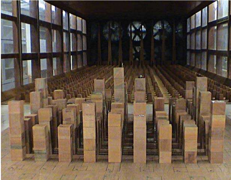
9.6. A scenario (random building height) inside the wind tunnel at NUS.
