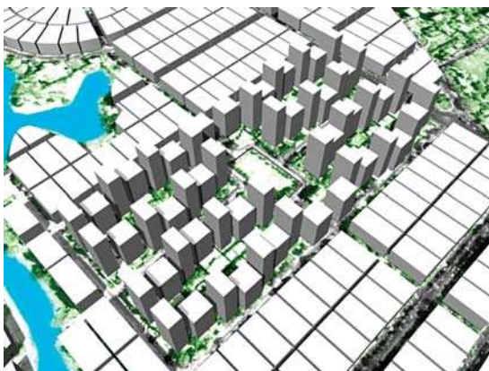
8.23. Application of FAR (allowing mixed of 50% and 66% open area with 12 and 18-storied height). (Source for Figures 8.21–8.23: Abdullah, A.Q.M., 2005)
